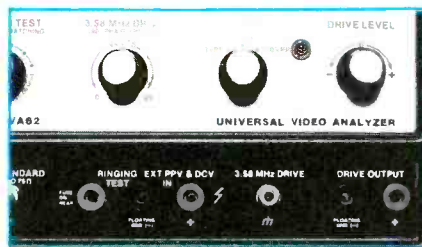
Figure 13 All VA62 cables exit along the lower part of the front panel which is black with white lettering. Jacks in this lower-right-corner area include those for the ringing test, the external PPV and dcV tests, the 3.58MHz drive, and the drive-output. Notice that the ringing, meter and drive-output jacks are isolated from ground.
