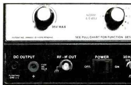
Figure 15 Jacks at the left bottom corner are for the internal dc-voltage supply. The RF/IF output jack is next, with the on/off power switch at the right.
