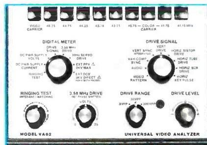
Figure 12 This photograph shows the controls in the lower right corner of the VA62 front panel. These include: the digital-meter selector; the drive-signal selector; the ringing-test impedance selector; the 3.58MHz drive amplitude control; the 3-position drive-range switch knob; and the zero-center drive-level rotary control.
