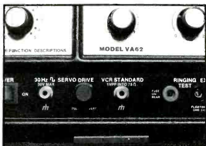
Figure 14 Signals exiting from jacks near the lower center of the panel include the 30Hz servo signal (with its amplitude control at the right), the VCR standard video patterns, and the ringing flyback-and-yoke test.
